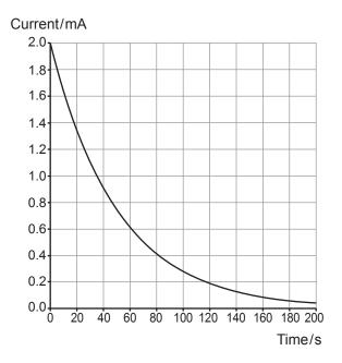
The switch is closed, and the capacitor allowed to charge fully. The switch is then opened at time t=0 seconds and the capacitor allowed to discharge through R. The graph shows how the reading on the milliammeter changes with time.
